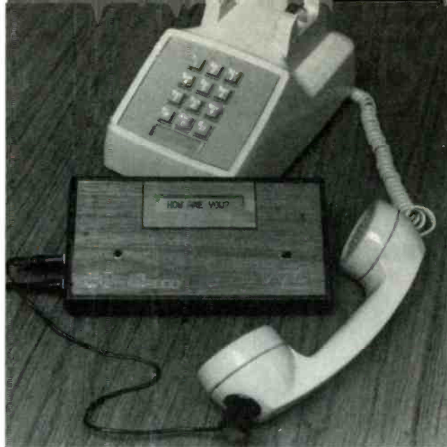
This battery-powered device enables deaf people to use a telephone anywhere—even in a public booth. At the deaf person's end of the line, the varying tones generated by the caller's push buttons are translated by special decoder circuits into letters that flow across the device's liquid-crystal display window in ticker-tape fashion.
