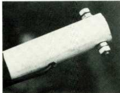
Fig. 2—Antenna wire terminals and coax feed-through at top of PVC mast.
