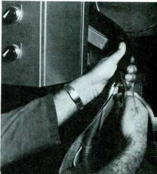
Fig. 2—One technique for shielding wires and cables from the effect of an EMP is to shield it with a product known as Zippertubing. The product's outer material is conductive.
