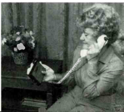
Stephen Fowler communicates with his deaf mother, Mrs. Sue Fowler (right), by tapping the keys of a push-button telephone. A device attached to his mother's phone provides a ticker-tape read-out on an LCD. Edwin Underkoffler (standing left), a GE computer specialist, is the inventor.
