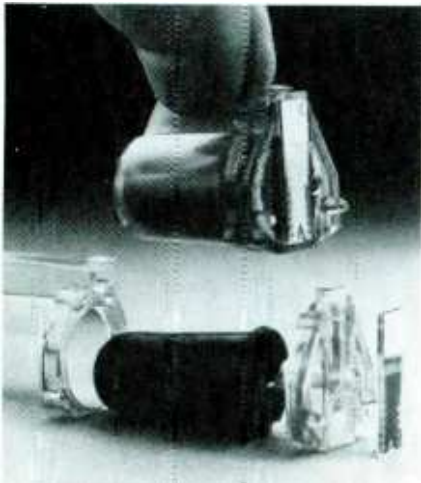
The printhead for the H-P Thinkjet personal printer is conveniently disposable and easy to reload. That design technique eliminates the necessity for clearing clogged jets.
