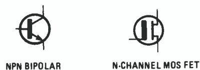
Fig. 7—Two of several transistor types used in binary circuits.
